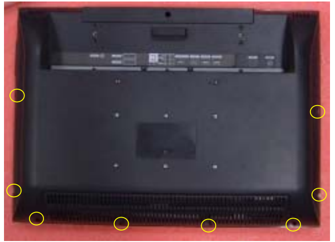
2. Release 8pcs screws from rear cover.
