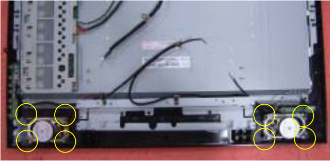
13. Release 8pcs screws from speakers.
