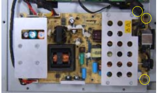
6. Release 7pcs screws from shielding.
