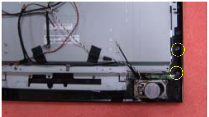
10. Release 6pcs screws from PCB tray.
