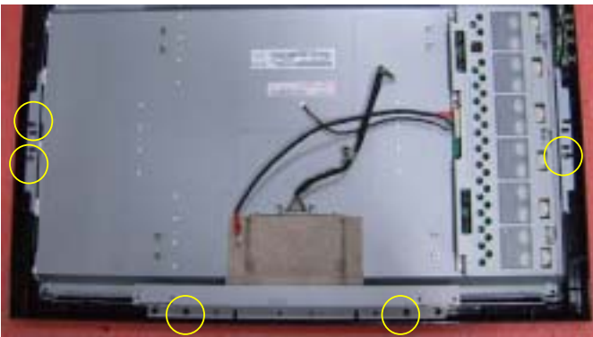
17. Release 5pcs screws from panel.
