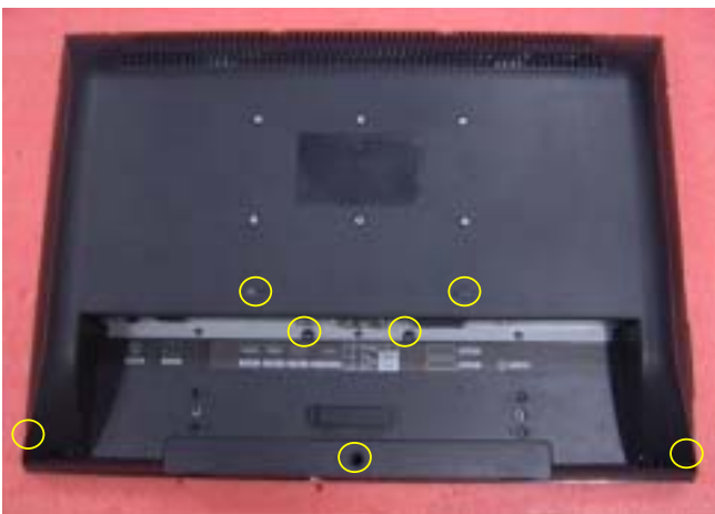
3. Release 7pcs screws from rear cover.
