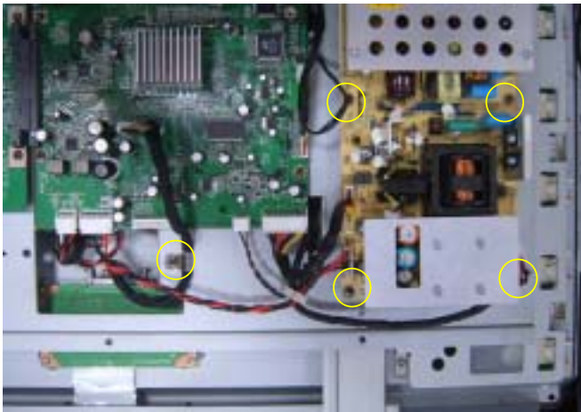
7. Release 5pcs screws from Power/B and GND cable.
