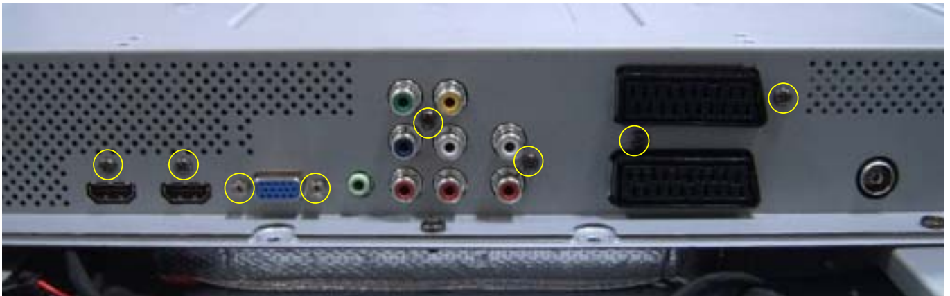
4. Release 8pcs screws from joint.
