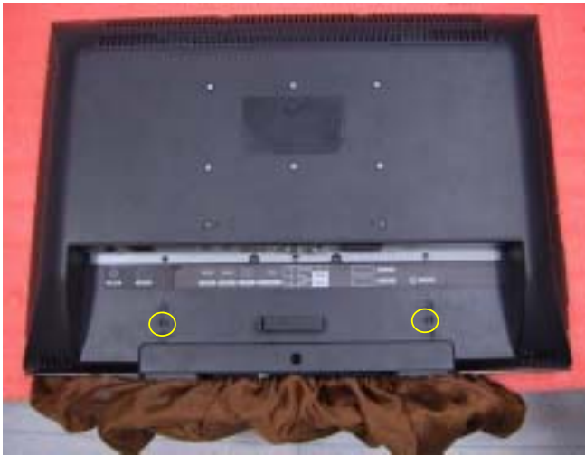
1. Release 2pcs screws and take off the base.
